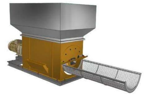
quickly as the size of the peanuts change. Directly driven by its motor and gear reducer, the shelling cylinder will start up under load.
