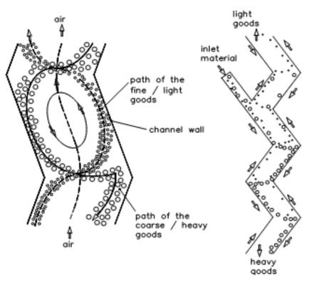
returned via blower to the separator base. In case of dusty or moist products the operation of the plant is also possible in partly air circulation or suction mode. The required air flow and pressure is generated by a radial blower.
